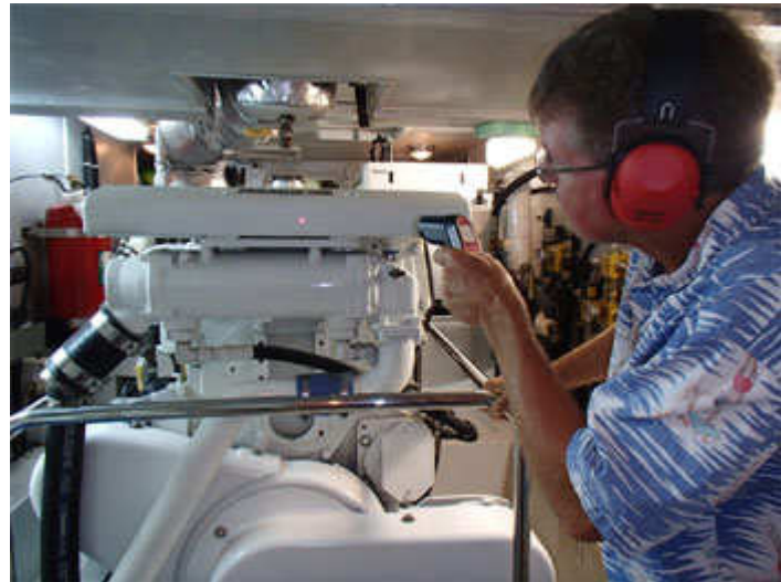
The author doing an engine room check with infrared thermometer gun (note ear muffs for sound protection).
