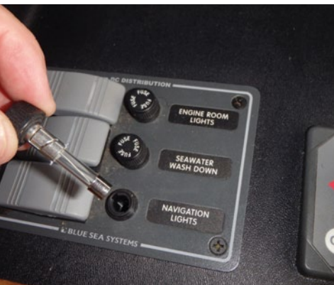
Above, make sure you have the right fuses for your gear. Right, spare fuses ready to go. Bottom, good labeling helps.
