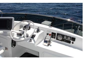
Flybridge steering station on a power voyager. Without sails to help balance the vessel, steering systems must be highly reliable. key components you should monitor as part of your regular maintenance routine; oil reservoir, hydraulic cylinder, hydraulic ram, tiller arm, oil manifold, rudder post, rudder bearings, etc.
