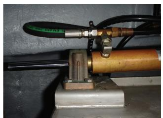
important. Regularly confirm that all of the connections that run the length of the rudder column up to the bearing in the rudder box are free from showing signs of wear and tear.
