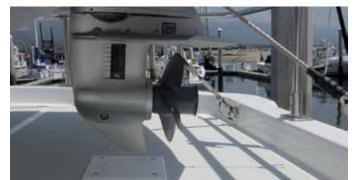
An outboard skid pad protects the deck from getting mared by the outboard's lower unit. "skid pad" below the skeg of the outboard to prevent damage to the deck and bottom end of the outboard.
