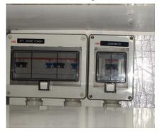
Shore power and generator breaker boxes located in the engine room of a power voyager.
