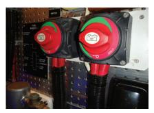
Make sure your battery selector switches are set properly for the situation, whether it be charging the house bank or the engine start batteries.
