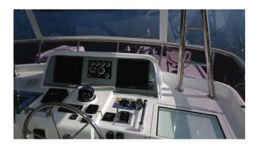
**Most flybridges** have a duplicate set of instruments and controls.
