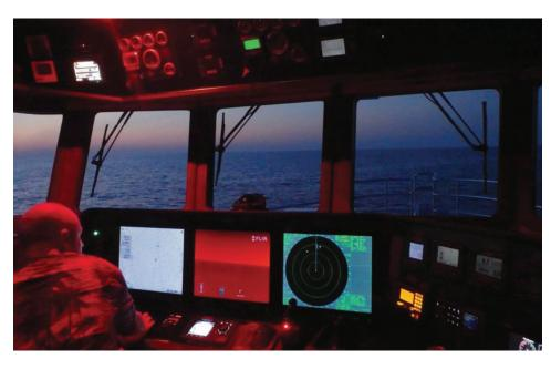
Above, a modern pilothouse with multiple screens can put out considerable light. Dimming the screens helps preserve your night vision. Right, a tidy instrument cluster on a Selene 59.
