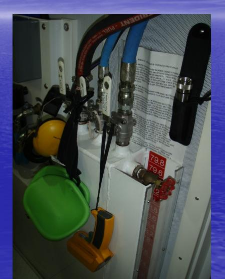
Engine Room Inspection \*Close the ER door (quiet and heat) \*Inspect Fuel valves – correct? \*Bilge water level – "tide stick" \*Temperature of stuffing box? \*Under Engine Drips? Belt Chafe? \*Racor vacuum gauges? \*Inspect all sight glasses
